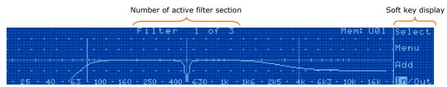
The display for the filters is similar to the home page, showing the frequency response - in this case just for the filters. At the top is a legend that indicates which filter is currently active for control and also how many filters are in use. So, for example, if we have three filters in use, and are adjusting the second one the legend would read "Filter 2 of 3". If no filters are active, then the display is blank except for the ADD key. Press this key to add a filter.
